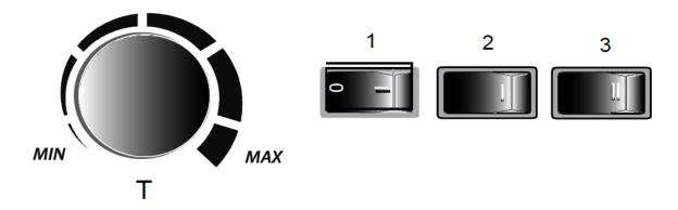
To maintain a certain room temperature, set the thermostat (T) to "Max". Operate the heater on full power until the required room temperature is reached, then turn the thermostat knob towards "Min" until it turns off with an audible clip. This temperature will be kept almost constantly by the thermostat switching the heater ON and OFF automatically. Please note the heater can only be switched ON when the thermostat setting is higher than the room temperature.
